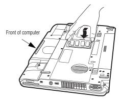
(Sample Illustration) Inserting the memory module into the slot
